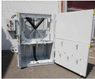
Low overall height and large feed opening for greater flexibility, ease of use and reduction in required labour.
