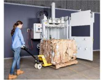
Large bale, designed with dimensions to fit on a standard pallet, improving supply chain efficiencies.
